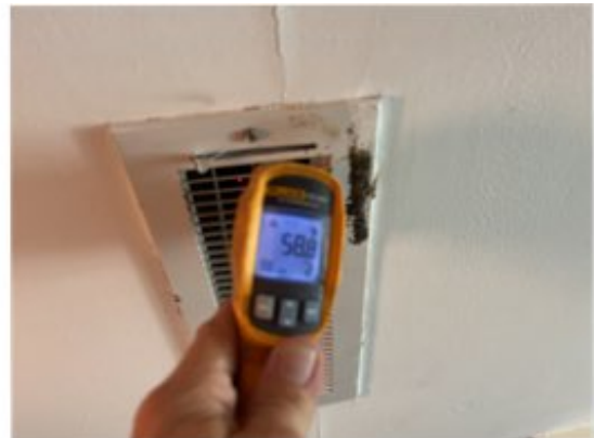
SECOND FLOOR REGISTER SUPPLY AIR TEMP
