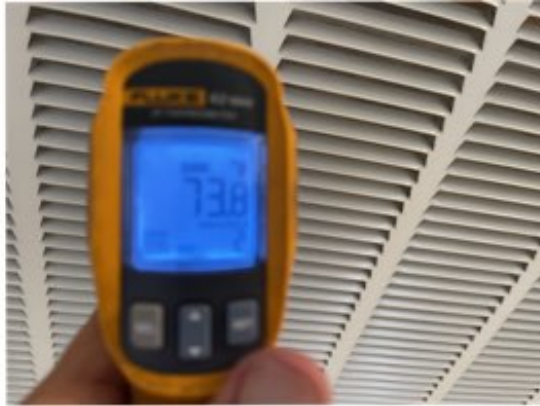
SECOND FLOOR RETURN REGISTER AIR TEMP
